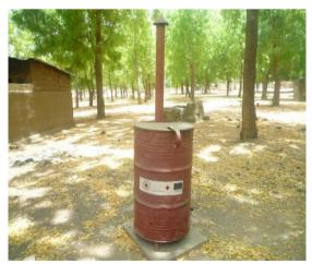
Figure 6: Local incinerator for Syringes
